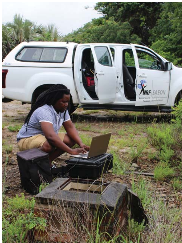
SAEON technician, Sipiwe Mfeka, downloads groundwater data from a monitoring sensor. Working in collaboration with various stakeholders, SAEON has established a network of groundwater monitoring sites which it maintains to determine trends in ground water dynamics and how this links to lake level, climate and different land uses in the region.
